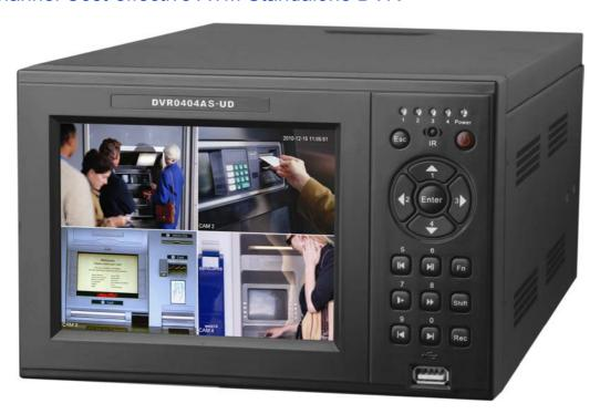
**TS-DVR04AS-U**: 4 channel video inputs and 4 channel audio inputs. The 1st video channel can support max D1(4CIF) realtime recording and other channels can support CIF realtime recording. It can support TV, VGA, and USB2.0.
