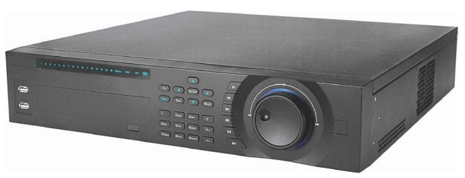
**TS-DVR32HF-S**: Full D1 recording, 32 channel video inputs, 16 channel audio inputs and 1 channel spot output with multi split display. It can support HDMI, VGA, eSATA, USB2.0 and 8 HDDs.
